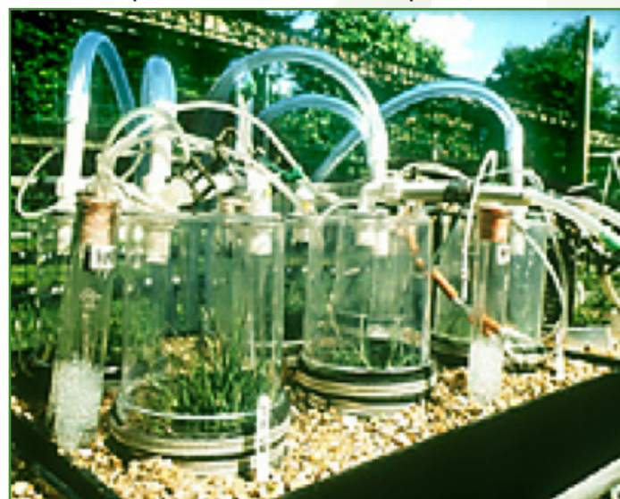
Measuring carbon flux in the Phoenix Lab
